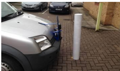
1m long pole in front of a camera mounted at 0.6m
